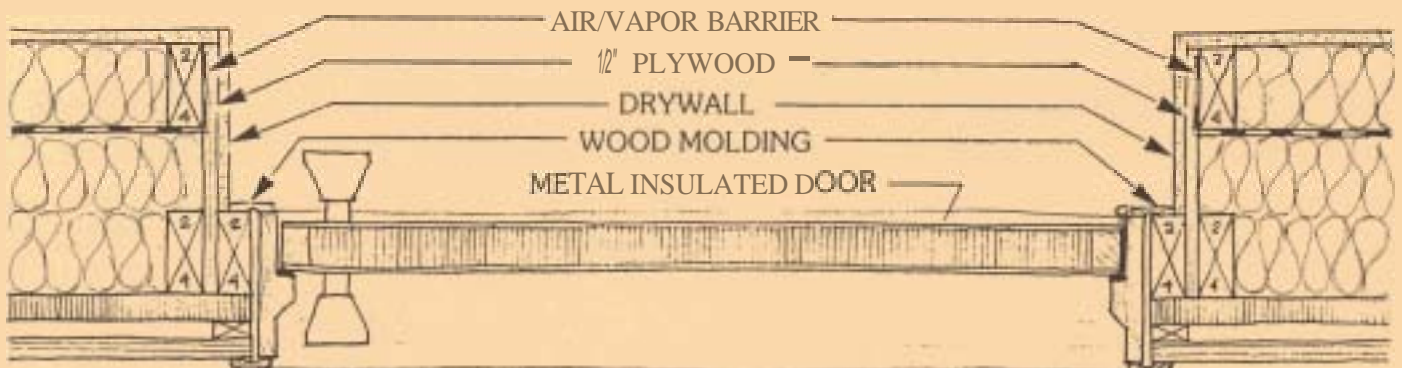
Detail 21 Door Installation in Double 2x4 Wall
